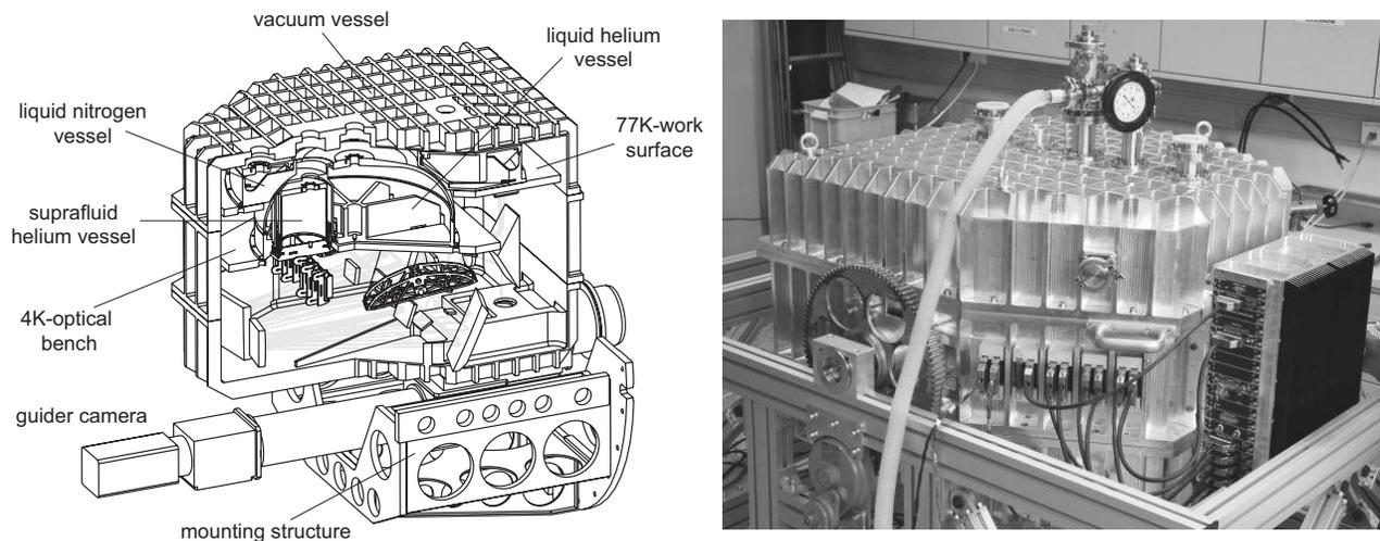
**Figure 1.** A schematic cut through the FIFI LS cryostat (left) and a picture of the actual instrument in the laboratory during a cool down (right).
