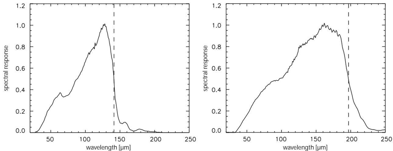
**Figure 5.** Typical relative spectral response of a low stress (left) and high stress (right) detector pixel. The peak response both curves is normalized individually. The dashed vertical lines mark the wavelengths of 50% response decrease, defining the cut-off wavelength.
