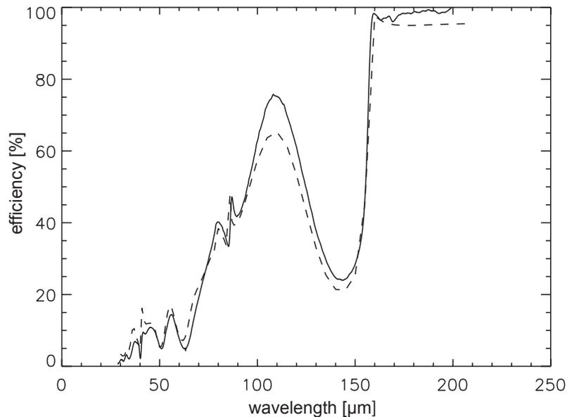
**Figure 4.** Measured and calculated efficiency curve of the long wavelength grating in  $0^{th}$  order. The solid line shows the measurement, the dashed line the result of a calculation using PCGrate.
