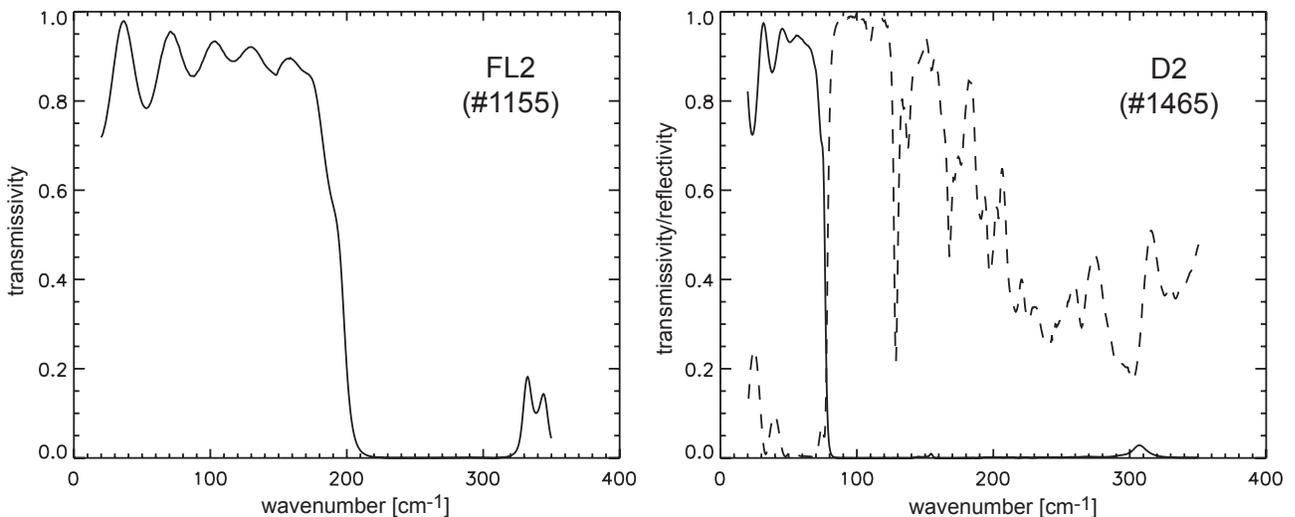
**Figure 2.** Typical filter curves of filters used in FIFI LS (compare Table 1). Left: Transmissivity of filter FL2. Right: Transmissivity and reflectivity of dichroic D2. Transmissivities are shown in solid lines, reflectivities in dashed lines.
