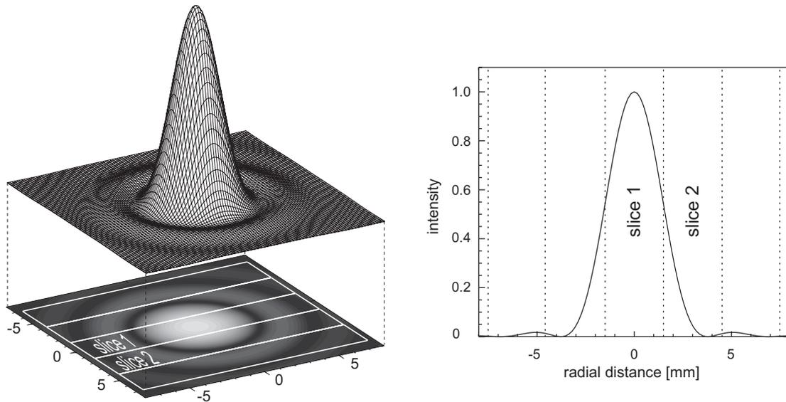
**Figure 7.** The image of a monochromatic ( $160 \mu\text{m}$ ) point source at the slicer mirrors of FIFI LS. Left: Three dimensional representation of the diffraction pattern (Airy function) and the projected intensity. The white rectangles represent the individual slicer mirrors and show how the mirrors cut into the Airy disc. Right: The intensity as a function of radial distance. The dotted vertical lines indicate the width of the individual slicer mirrors.
