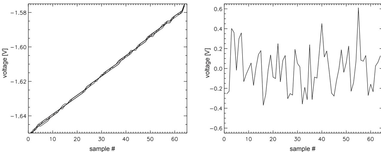
**Figure 6.** Left: Typical integration ramps measured with a blackbody temperature of 35 K. Right: One of the ramps of the right panel after subtraction of the average ramp slope.
