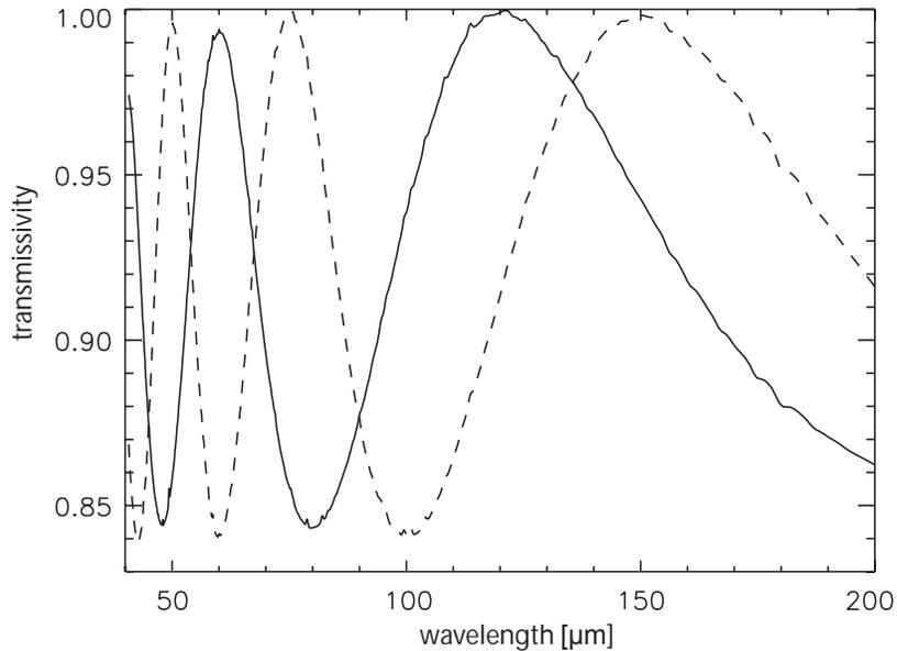
**Figure 3.** Transmission curves for 40  $\mu\text{m}$  (solid line) and 50  $\mu\text{m}$  (dashed line) polypropylene foil used as window material for FIFI LS.
