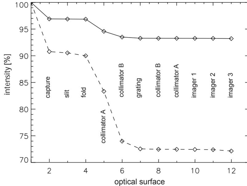
**Figure 8.** The light loss through the long wavelength spectrometer (for  $160 \mu\text{m}$ ) due to diffraction effects and vignetting by the indicated optical surface. The solid line shows the light loss through the central slice, the dashed line through the first off-center slice respectively.
